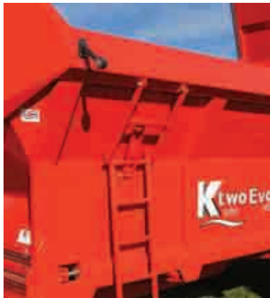
Splayed side walls
